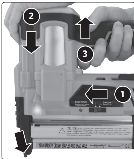
Fig. 4, single shot mode (selective contact triggering)
